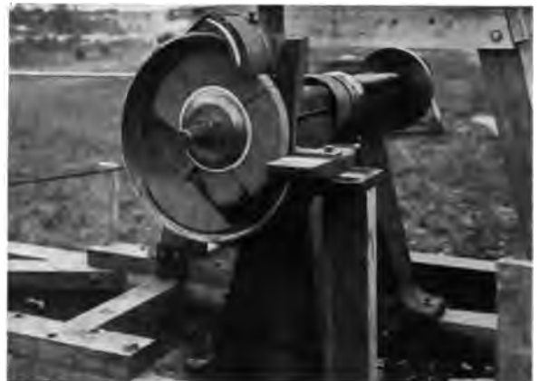
Fig. 3. Test of Hood showing its effectiveness in retaining parts of broken wheel.
